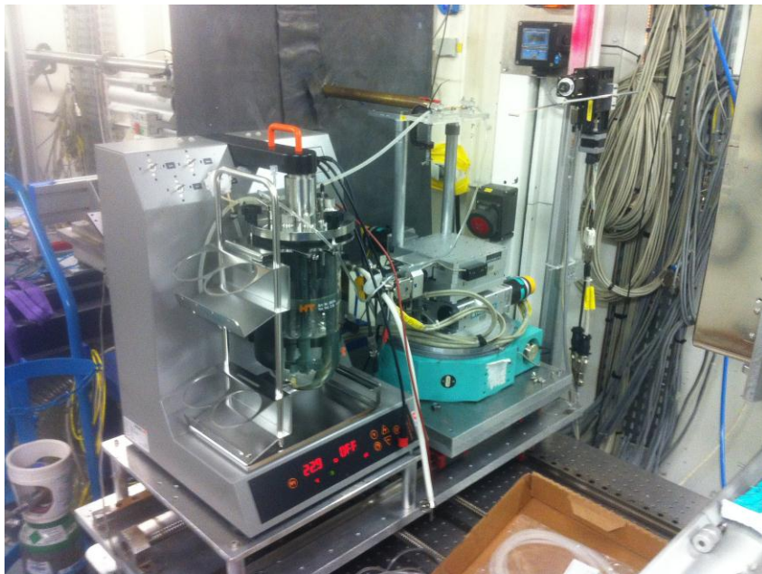
Portable chemical reactor installed at beamline ID15 (ESRF) for in situ synchrotron experiments
